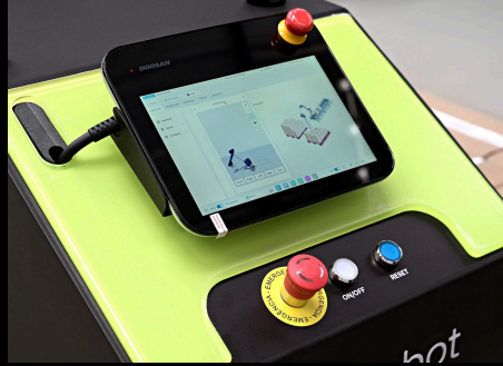
Operator touch screen. Recipes and pallet patterns are selected directly by the operator, without robot reprogramming.
