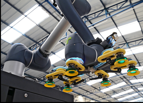
Vacuum gripper. Selected for your case type, size, weight and surface; clamp tooling is also available.
