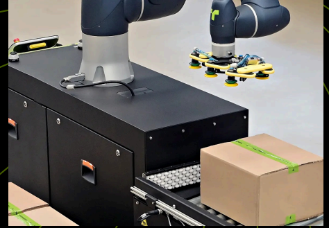
Infeed and pick point. Cases arrive on the infeed conveyor and the robot picks each one for the programmed pattern.
